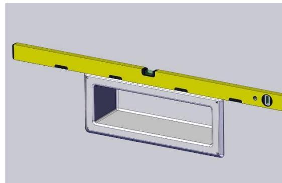
2. After the holes are marked and the anchors are in, fit the shelf in the opening and make sure it is level.
