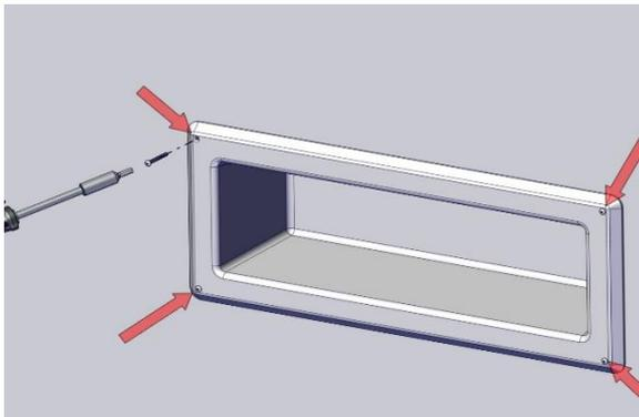
3. Screw the shelf to the wall in the pre-installed anchors
