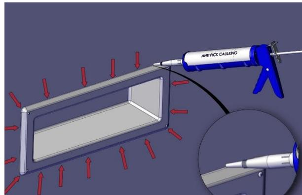
4. Put a bead of anti-pick caulking on the flat edge of the shelf.
